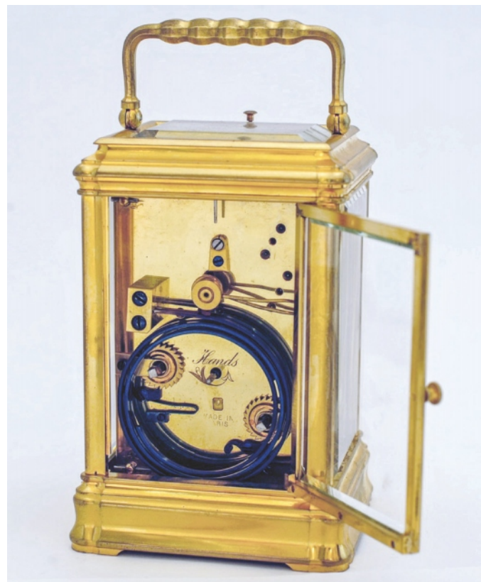
Figure 10, left. Albert Jacot serial no. 14850. Grand sonnerie and repeat on a gong. Gilt-brass gorge case. Jacot stamp. Award date 1889. USED WITH PERMISSION FROM A PRIVATE COLLECTION.
